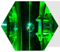
Scientists use a laser to measure the temperature and density of the plasma created at the Proto-Materials Plasma eXposure Experiment. The facility is used to test materials that could protect the plasma-facing walls inside fusion reactors.
