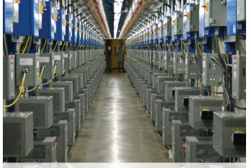
The 120-machine Commercial Demonstration Cascade has achieved more than 20-machine years of operations.
